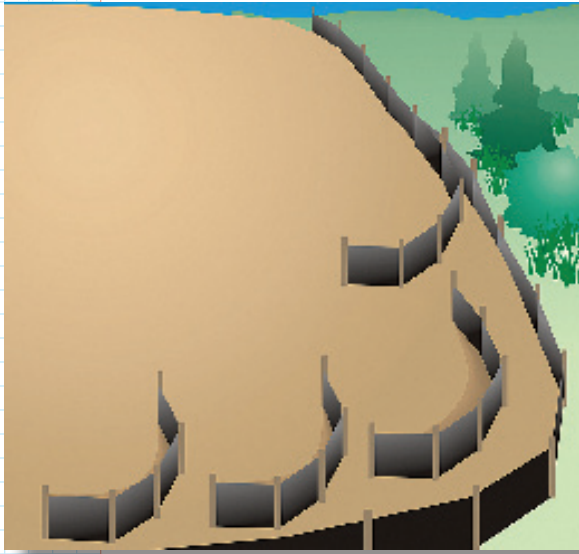
Use several short lengths of silt fence and J-hooks to intercept converging runoff in critical areas, such as property corners. This can help relieve stress and prevent failure at the corners.
