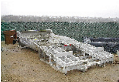
This is a commercial concrete washout tank with fold-up ramp.
