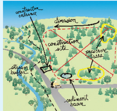
Identify drainage areas and drainage ditches and channels. Install diversions, grassed channels, sediment traps/basins, downslope sediment barriers, and rock construction entrance before beginning work.
