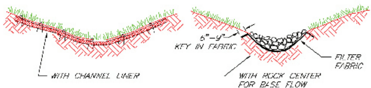
TYPICAL PARABOLIC CHANNEL CROSS SECTION
